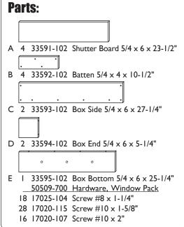
All hardware on this set is specially coated for corrosion resistance. If non-Creative Playthings hardware is used, it must be galvanized or stainless steel.
