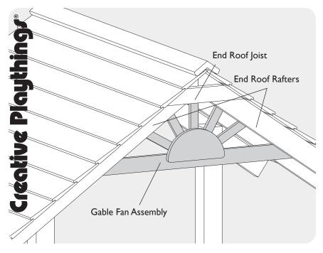
All hardware on this set is specially coated for corrosion resistance. If non-Creative Playthings hardware is used, it must be galvanized or stainless steel.
