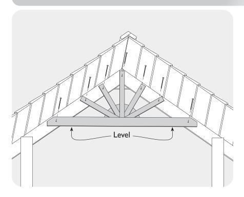
Before installing the Gable Fan Assembly, make sure that the End Roof Joists are mounted to the outside of the End Roof Rafters.
